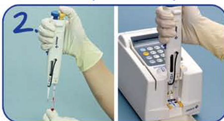
Draw the sample and reference solution with the Twin-pipette. Set pipette and apply sample to E-plate
